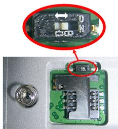
A slide switch is available at the bottom of the battery compartment to set the behavior of the receiver after removal or failure of the DC power source while the receiver is on:
