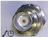
**GNSS Input #2 Option.** A TNC coaxial female connector [8] for a second GNSS antenna input (future optional heading mode), or for applying an external reference clock. (Connector [8] is missing from the rear view above.)
