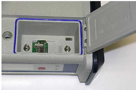
The battery used is a 7.4-V DC - 4400 mAh rechargeable battery. It is a standard model used in many camcorders. The battery is housed in a battery compartment accessible from above the ProFlex 500. The compartment door can be opened by lifting and then turning the quarter-turn finger screw counter-clockwise.
